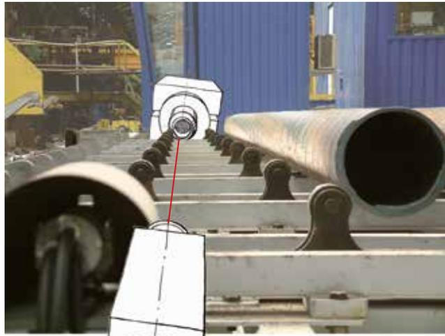
Length measuring of pipelines - transversal transport
