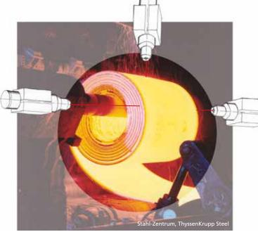
Determination of coil diameter
